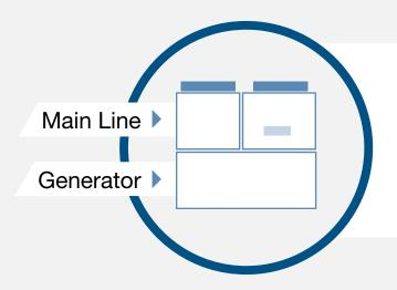
With the double power supply configuration, the unit is equipped with an ATS (Automatic Transfer Switch) and can be connected to two separate power lines (usually the mains and the auxiliary generator line). In case of a main line power outage, the ATS automatically switches over to the other line, granting uninterrupted power supply to the unit.
