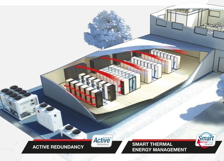
A real active redundancy achieved through the adoption of innovative EC PUL fans together with Inverter DC brushless compressors (on direct expansion units) and an advanced algorithm for balancing the heat loads among the units (including those units that usually remain in stand-by).
