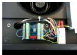
Morsettiera interna Internal terminal (Termostato/Thermostat)
